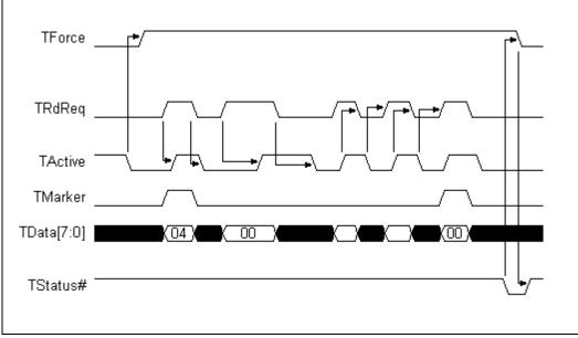
Figure 1. TCO Timing Diagram
