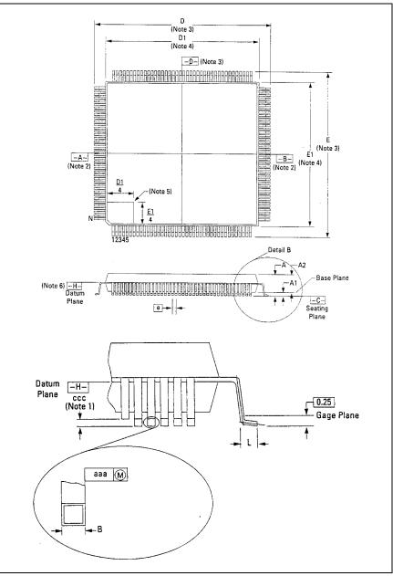
Figure 3. Dimension Diagram for the Alert on LAN ASIC
