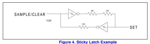
*Note:* This solution also prohibits the use of the ASIC cover tamper clear mechanism (the ASIC can be configured to output a 20 ms clear pulse). The environmental IC should clear the sticky latch.
